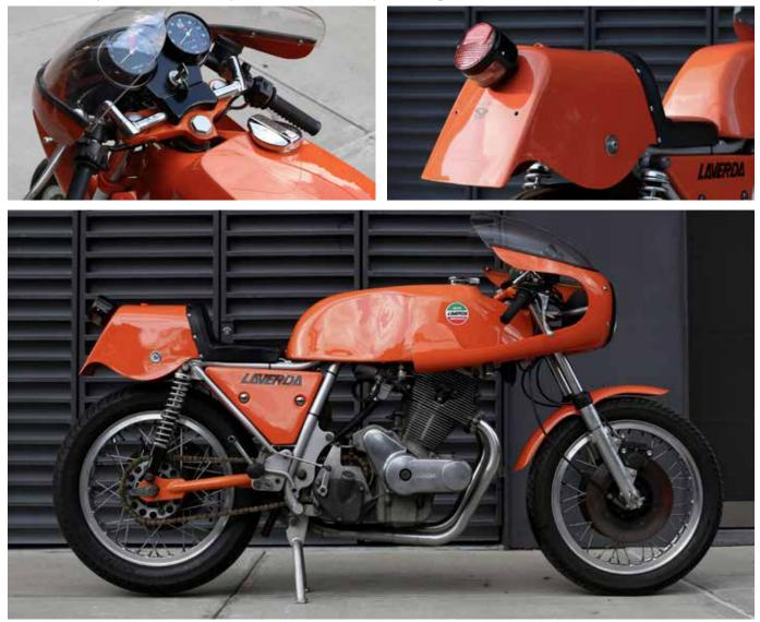
Two of the most significant updates for 1974 was the pair of Dell'Orto PHB 36 carburetors, without accelerator pumps, and twin-bleed Brembo F08 calipers with twin front discs, and a single rear disc on an Elektron hub. A racing two-into-one megaphone (as on this example) accentuated the lean race replica profile, and the claimed power for the 1974 750 SFC was 75 horsepower at 7,500 rpm. The right-side gear shift remained as did Borrani rims and Ceriani suspension front and back.
