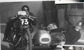
Hans Stärkle, on right hand side, with a customer in front of his workshop, c.1950. RC3548 can be seen fitted with large size wheels, manual ignition, altered seat for sidecar use, large rear sprocket, also for sidecar use, and solid rear end.
